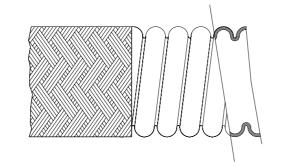
**SERIES HC** is a heavy wall extruded convoluted hose used extensively through the process industry. It's self cleaning design and unique way the hose can be lined through the fittings makes a completely bug free environment for applications where cleanliness is paramount. This also protects fittings against corrosion in applications transferring aggressive medias.
